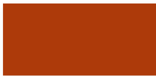
Terra Cotta SR: .35 E: .87
